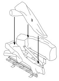
Figure 48 - Installing Log Assembly No. 3
